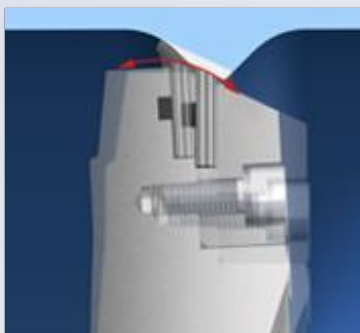
Triple offset design guarantees a frictionless swivel movement of the sealing ring into the seat
