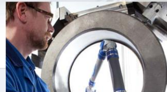
The three-dimensional measuring system allows the comparison with 3D data
