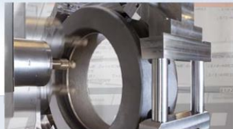
The valve bodies are manufactured on fully automatic, CNC controlled machining centres
