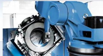
Fully automatic welding robot with an integrated measuring system
