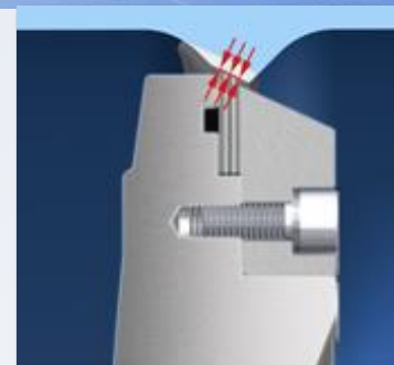
The ZETRIX® seals according to the area seating principle; the required contact pressure is applied via the actuator
