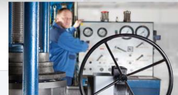
Computer aided leak test according to DIN EN 12266, leakage rate A
