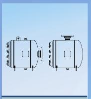
Ball float steam trap with inside strainer and pilot operated for steam range
