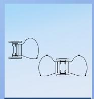
Ball float steam trap with inside strainer and pilot operated for steam range
