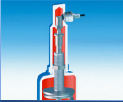
Integrated proximity switch (feedback signal returned to control room for example)
